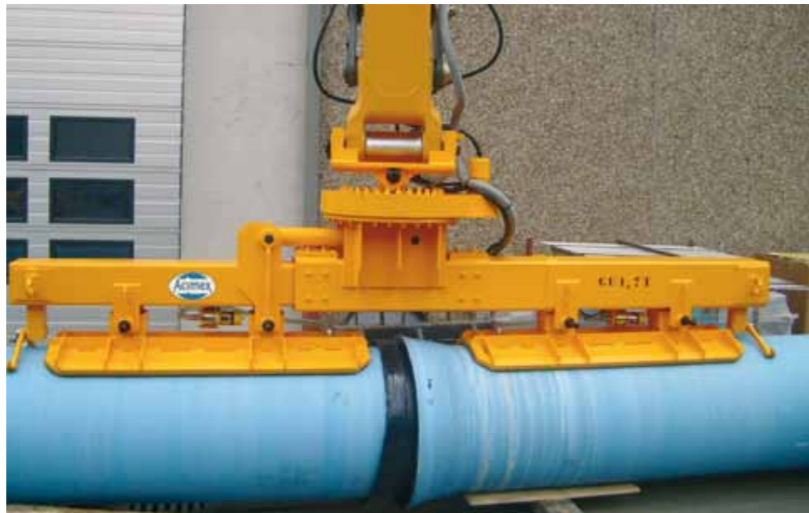
Vacuum pipe lifter with coupling system - SWL: 1.7T - DLE Company
