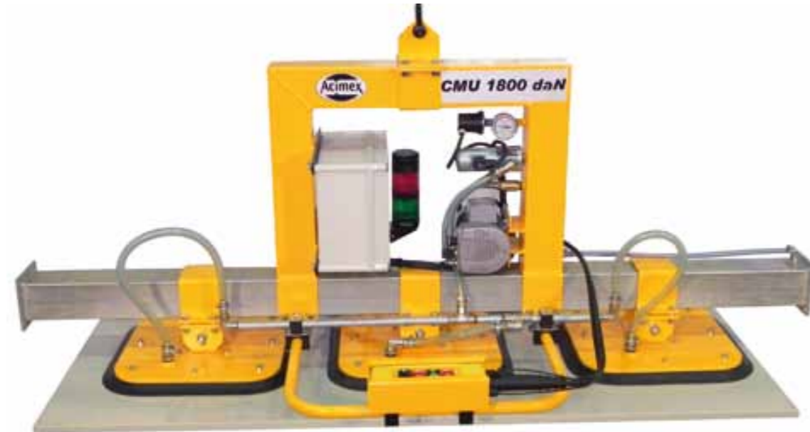
Modulift version for light steel sheets
