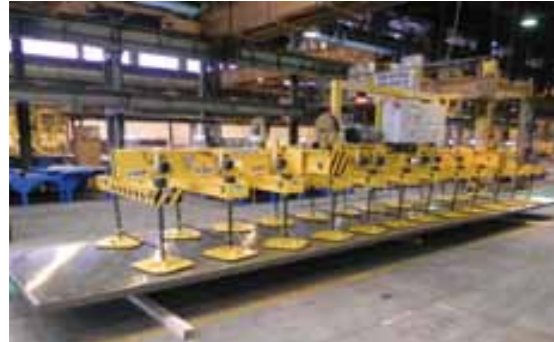
Vacuum beam for aluminium plate application - SWL: 9T
