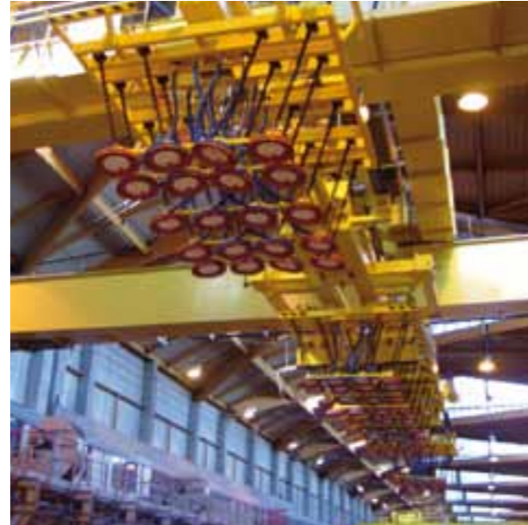
Upgradable vacuum beam for high temperature (300°) aluminium plates
