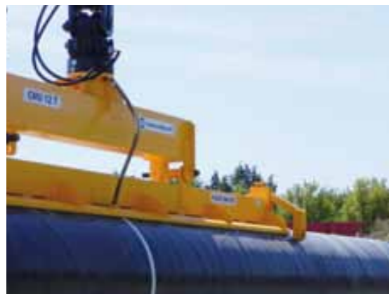
Vacuum pipe lifter for Liebherr excavator
