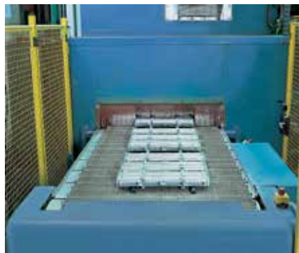
Installation de brasage CAB (Controlled Atmosphere Brazing)
