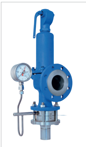
Fig. 2: Combination Device with a V-Series rupture disc for In-Situ Testing of Pressure Relief Valve.
