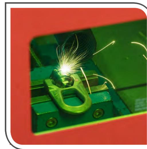
“ These lifting rings are certified and engraved with a safety factor of 5 which allows them to be used all over the world (including North America). CODIPRO also provides all information required for use with a safety factor of 4 as defined in EN 1677-1 standards. ”
